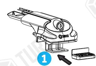
**EN** Attach the gasket that comes out of the box to the metal jaw as shown in the figure.
