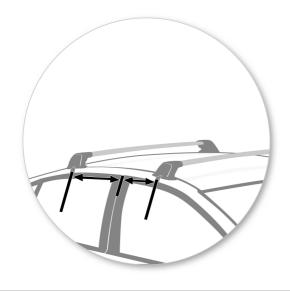
Place crossbar on vehicle. Minimum recommended spacing between the bars is 700mm (27 1/2") (unless otherwise stated).
