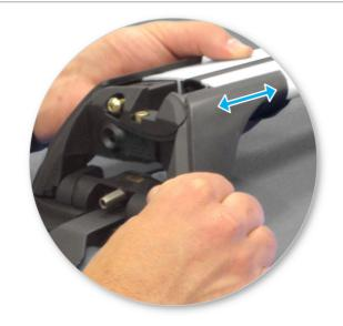
Adjust the legs on the crossbar so that they are positioned equally from the ends of the crossbar, and the clamps engage firmly on the body work of the vehicle.
