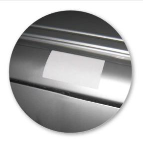
Apply masking tape to vehicle roof in all four positions.
