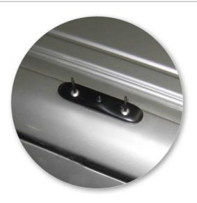
Install rivets through permanent mount blocks.
