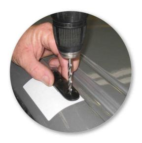
With the drill, lightly mark both permanent mount hole positions while holding the mount firmly on roof.
