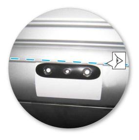
Position the permanent mount block so the inner edge of the block is on the outer edge of the ditch channel.
