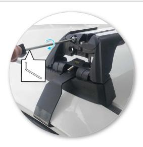
Tighten adjusting screw to 2 Nm (1.5 ft lb) hand tight.
