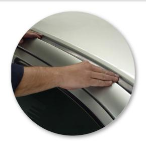
Re-install rubber ditch mould in roof channel.
