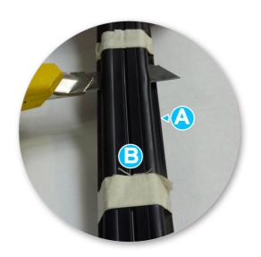
Carefully cut rubber ditch mould between faces along steel strip.
